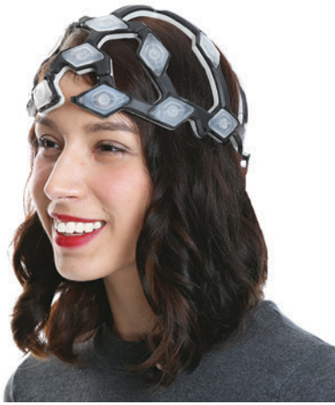
Fig. 1. The WAVi EEG device is a noninvasive method that tracks and records brainwave patterns
